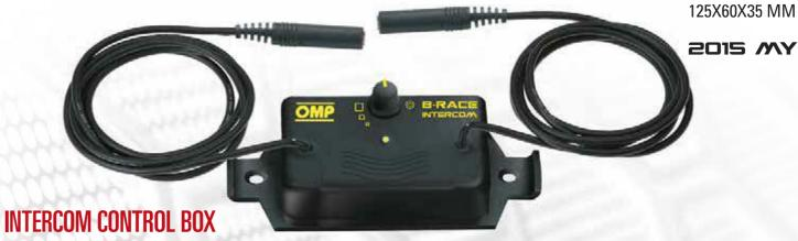
New components for improved sound quality. Without loudspeakers and microphone. One single driver/co-driver volume control. Powered by 9V PP3 battery (not supplied) or by car battery using JA/851 cable - can be fixed to rollbar and dashboard. Can be used with loudspeakers and microphone kit (JA/849, JA/854E) or headseats JA/850E.
