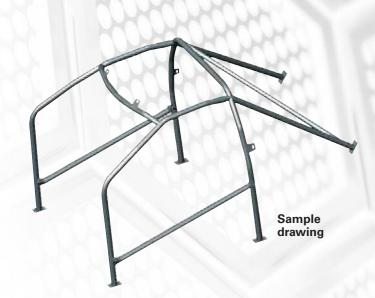
FE45 steel multi-point boltin roll bars with Ø 40x2 & 50x2 tubing, connecting sleeve tubes and door bars. To be cut to measure and welded upon installation.
