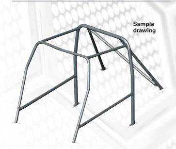
Off road Fe 45 steel bolt-in roll bars.
