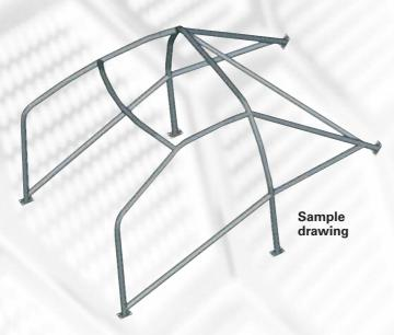
FE45 steel weld-in roll bars with Ø 50x2 tubing on the main hoop and Ø 40x2 tubing elsewhere. It may be necessary to remove or cut interior panels to facilitate installation.
